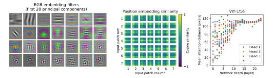
Figure 7: **Left:** Filters of the initial linear embedding of RGB values of ViT-L/32. **Center:** Similarity of position embeddings of ViT-L/32. Tiles show the cosine similarity between the position embedding of the patch with the indicated row and column and the position embeddings of all other patches. **Right:** Size of attended area by head and network depth. Each dot shows the mean attention distance across images for one of 16 heads at one layer. See Appendix D.7 for details.
