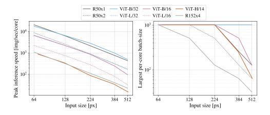
Figure 12: **Left:** Real wall-clock timings of various architectures across input sizes. ViT models have speed comparable to similar ResNets. **Right**: Largest per-core batch-size fitting on device with various architectures across input sizes. ViT models are clearly more memory-efficient.
